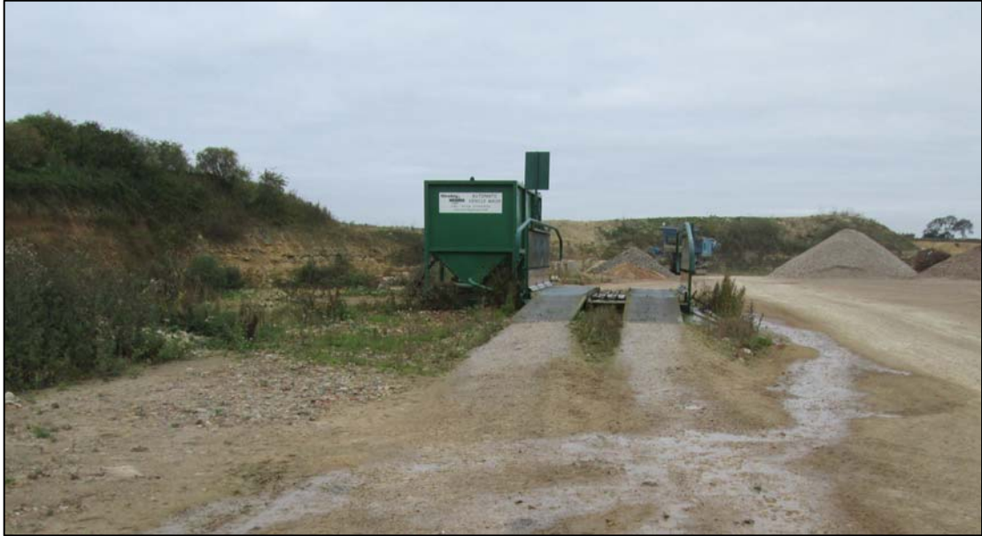
Photograph 2: Dunston Quarry Wheel Wash
